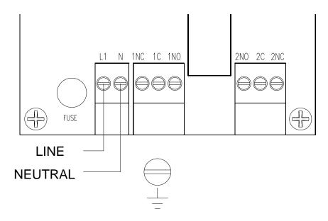
The FDC1000 control unit is powered from 120VAC 50/60Hz at 5VA. Wiring to the unit must comply with the National Electrical Code and local codes. A DPDT relay provides dry contacts for operation of auxiliary alarms or controls at the users discretion. These contacts are rated for 5A at 240VAC or 30VDC.
